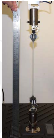
Shapes of the specimen before and during the tensile testing.
